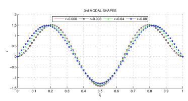
Figure 3. Third modal shapes for clamped-clamped beam
