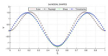
Figure 8. Third modal shapes for clamped-clamped beam
