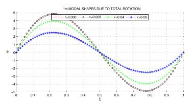
Figure 4. First modal shapes due to complete rotation
