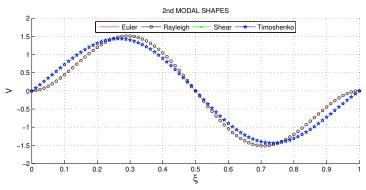
Figure 7. Second modal shapes for clamped-clamped beam
