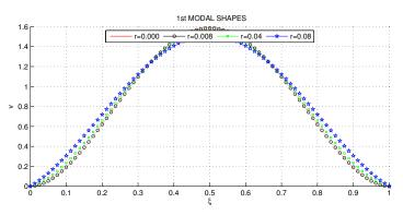
Figure 2. First modal shapes for clamped-clamped beam
