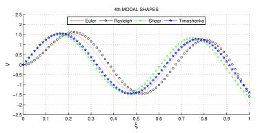
Figure 14. Fourth modal shapes for clamped-free beam
