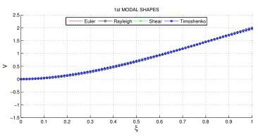
Figure 11. First modal shapes for clamped-free beam
