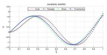
Figure 13. Third modal shapes for clamped-free beam
