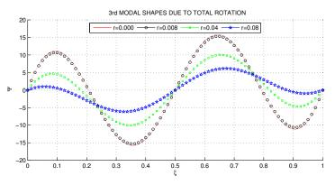
Figure 5. Third modal shapes due to complete rotation
