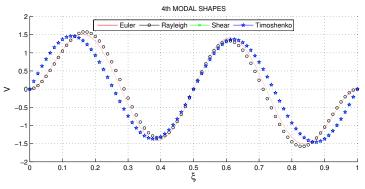
Figure 9. Fourth modal shapes for clamped-clamped beam
