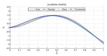
Figure 12. Second modal shapes for clamped-free beam
