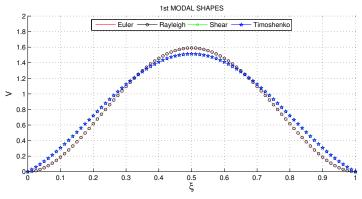
Figure 6. First modal shapes for clamped-clamped beam
